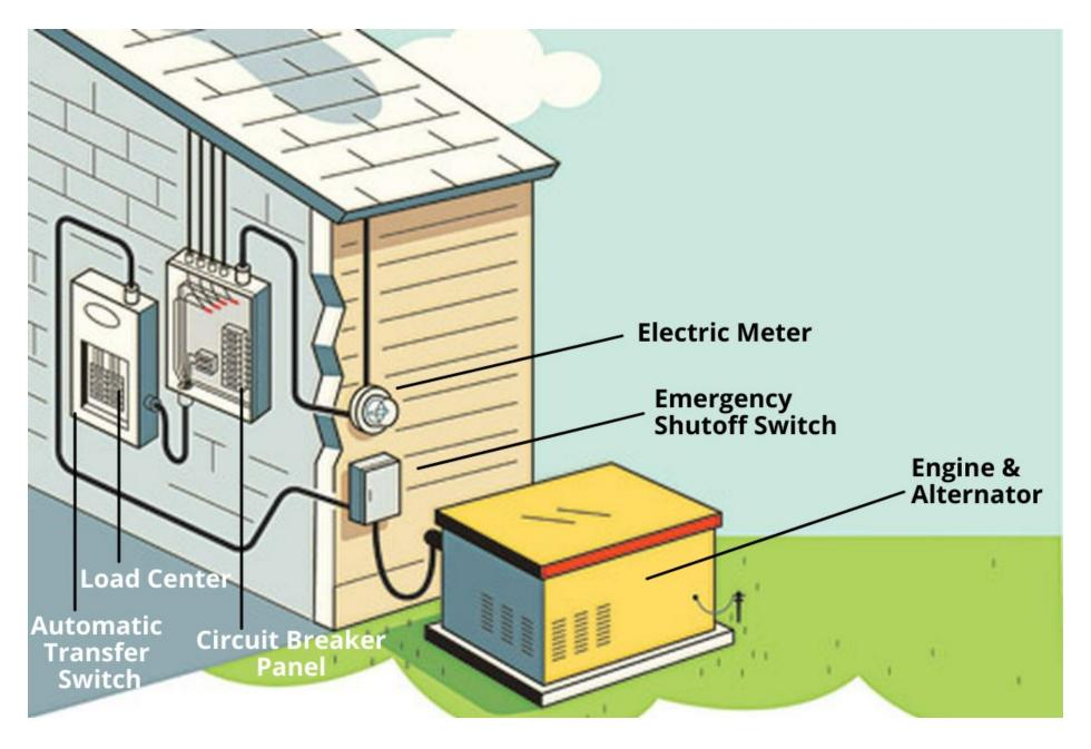
NOTE: 6-foot clearance required in front of and around the meter.
