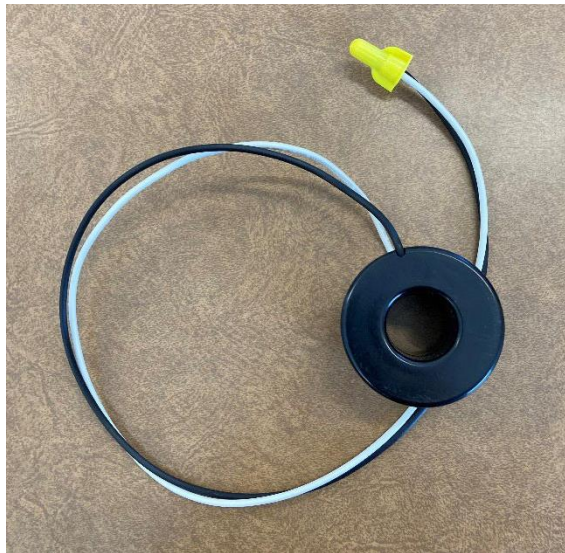
Current transformer – supplied by SCEC
