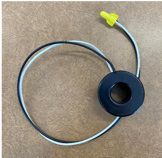
Current transformer – supplied by SCEC
